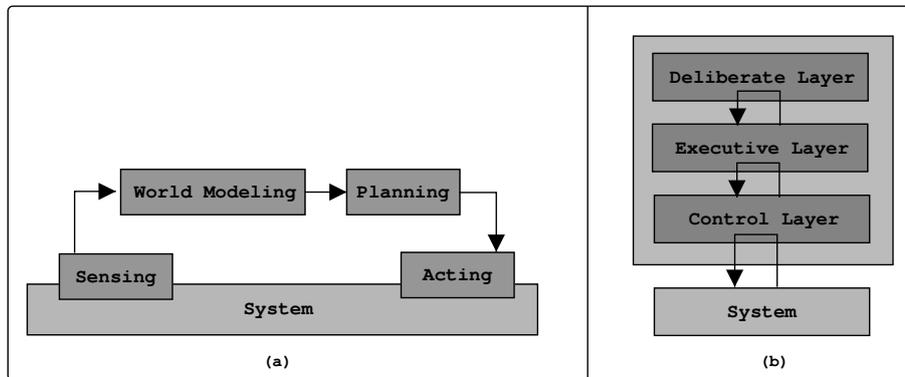
Figure 1.2: (a) *The “Sense/Plan/Act” open-loop*, (b) *The three-layered architecture*
