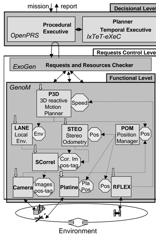
Figure 4.1: *Instantiation of the LAAS architecture on Dala*
