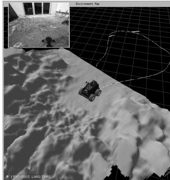
Figure 4.3: *Digital elevation map*
