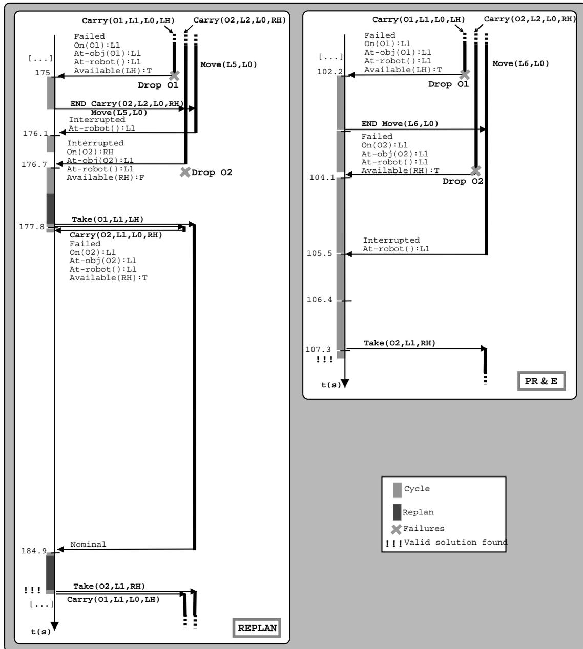
Figure 5.2: Reaction to a sequence of failures
