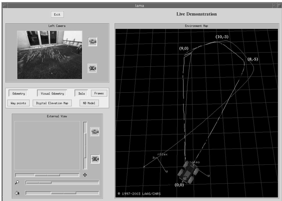
Figure 4.5: Path covered by *Dala* during Run 1. The trajectories labeled “*rflex*” and “*steo*” represent the position estimated respectively by odometry and visual odometry along the path. The visual odometry is indispensable even if it considerably slows down the robot.
