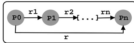
Figure 2.11: Conjunction of elementary resolvers
