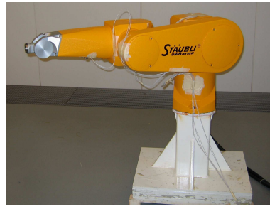
Figure 7: Flat configuration of a Stäubli Rx90
