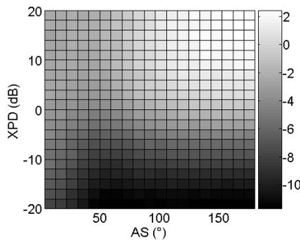
Fig. 3: Difference between the triple-polarized and the single-polarized channel capacity of  $4 \times 4$  MIMO systems in the functions of XPD and AS
