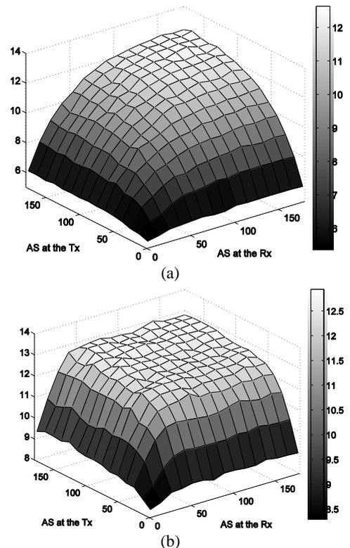
Fig. 2:  $4 \times 4$  MIMO channel capacity of isotropic antennas: (a) single-polarization system and (b) dual-polarization system
