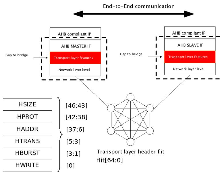
Figure 4.9: AHB end-to-end connection
