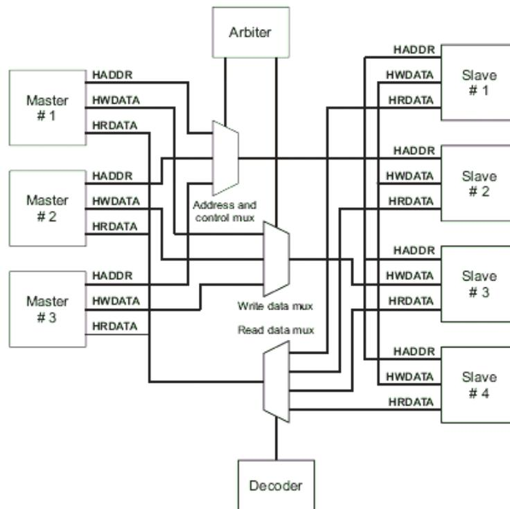
Figure 3.3: AHB bus microarchitecture
