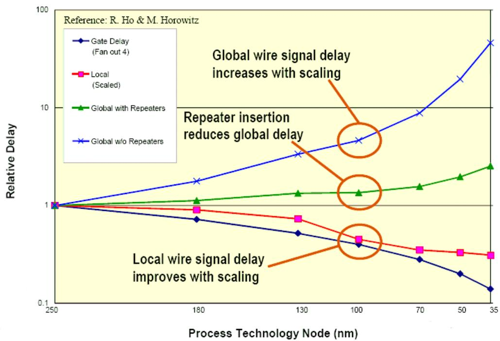
Figure 3.1: Local vs. Global wires delay
