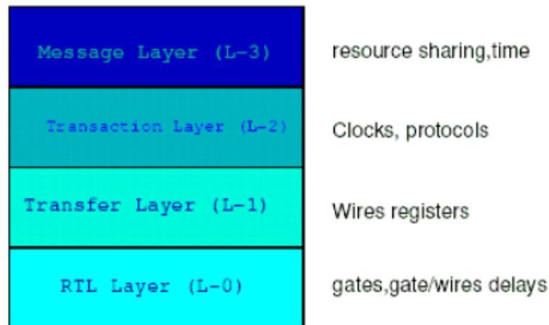
Figure 5.5: TLM stack of communication layers
