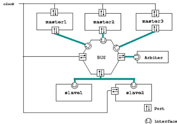
Figure 5.4: SystemC Simple Bus TLM structure
