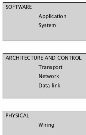
Figure 4.1: Adaptation to networks on-chip paradigm of OSI [63] stack
