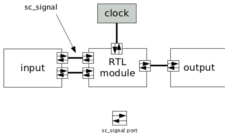
Figure 5.2: SystemC sample RTL model
