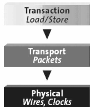
Figure 3.15: NoC layers in Arteris solution
