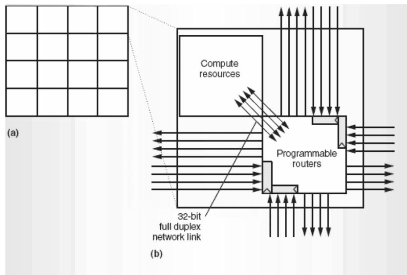
Figure 3.13: RAW on-chip interconnect a) RAW 16 tiles architecture b) Each tile has computational resources and four networks, each with eight point-to-point 32-bit buses
