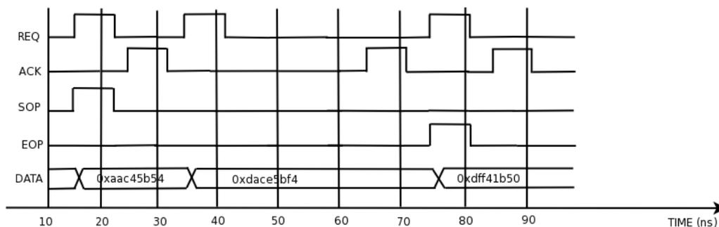
Figure 5.11: Standard router link protocol handshake
