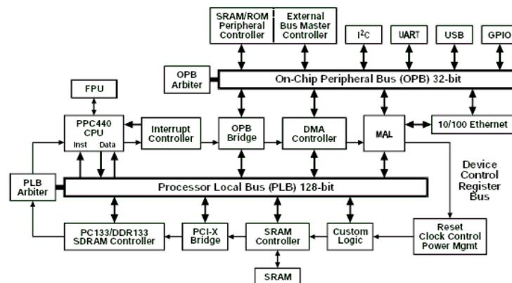
Figure 3.5: CoreConnect Based System-on-a-chip
