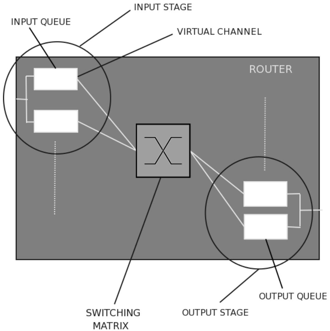
Figure 5.10: Standard router sketched micro-architecture
