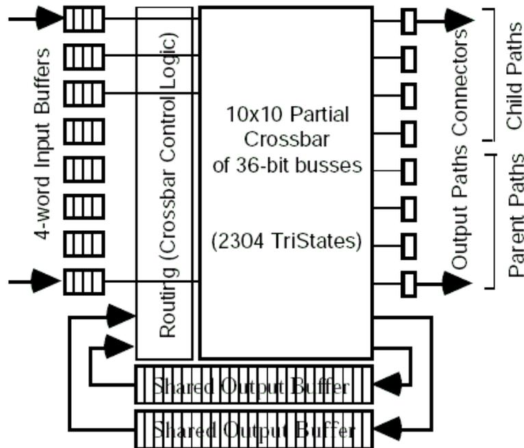
Figure 3.11: SPIN router macrocell microarchitecture
