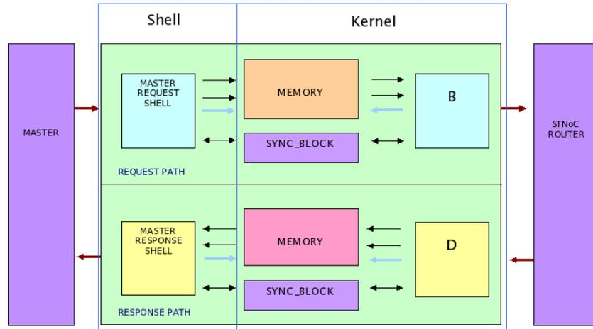
Figure 5.15: Mock-up of a NI microarchitecture
