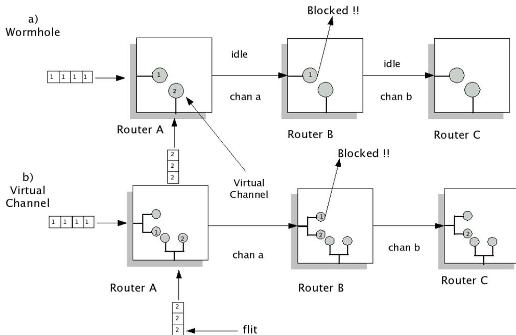
Figure 4.3: In wormhole flow control (a) Packet 1 blocks; channel a and channel b are idle even though packet 2 could exploit their bandwidth. In virtual channel flow control (b) 2 can advance by using a second virtual channel.
