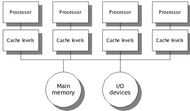
Figure 4.10: UMA multiprocessors architecture
