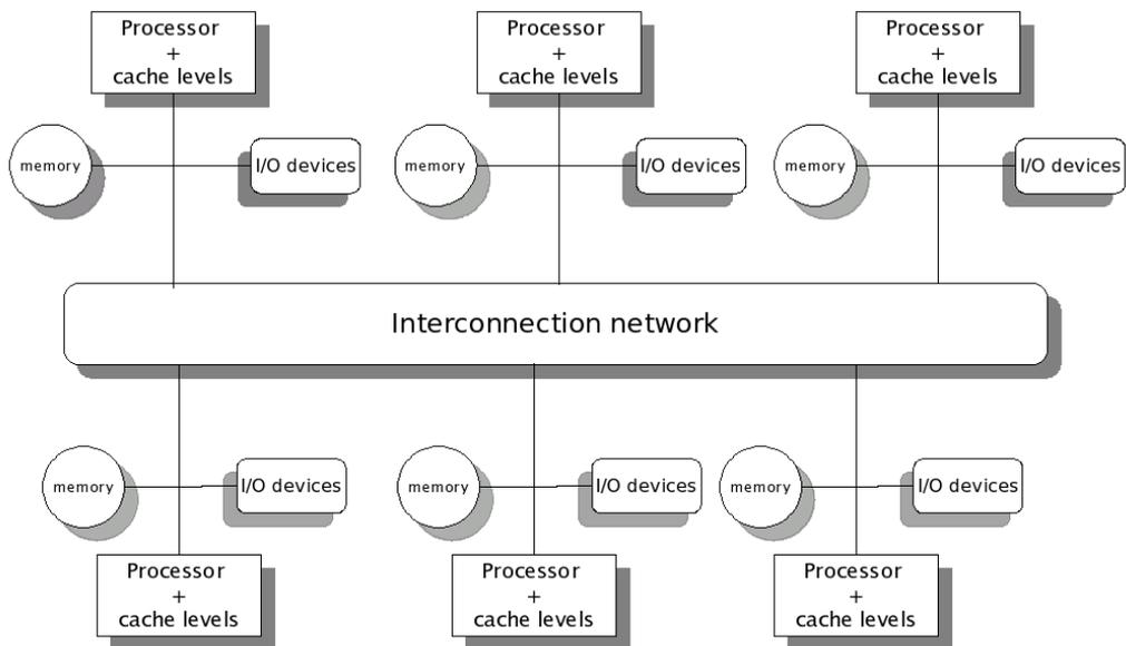
Figure 4.11: NUMA multiprocessors architecture
