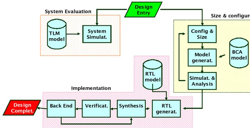
Figure 6.2: STBus genkit design flow
