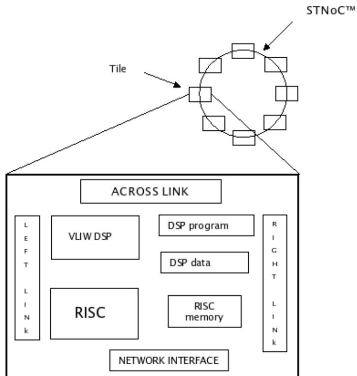
Figure 8.2: STNoC™ in a multi-tile parallel architecture
