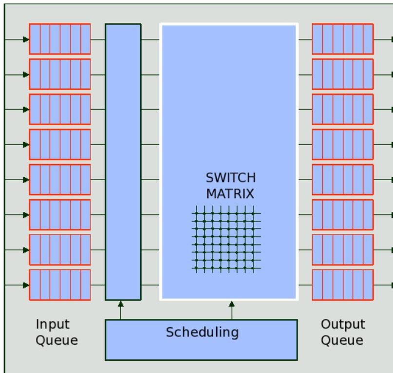
Figure 4.13: Generic NoC router microarchitecture
