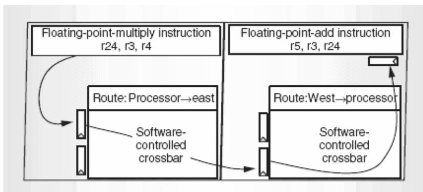
Figure 3.14: Two RAW tiles communicating over a static network
