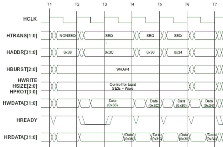
Figure 4.8: AHB wrap4 burst transaction
