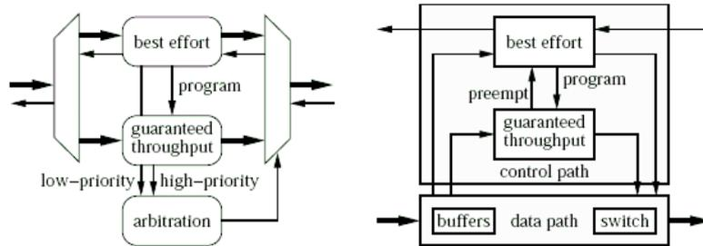
Figure 3.12: Overview of an Æthereal router
