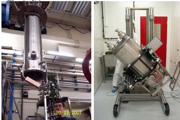
Figure 1: Cavity A and one of the 2 cavities B in the clean room with the handling robot
