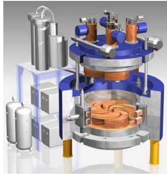
Fig. 11: Accel supraconducting cyclotron.
