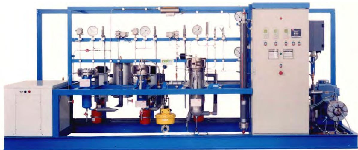
**Figure IV.2: Pilot plant scale supercritical drying apparatus of Natex, Austria. Photo courtesy of Natex.**
