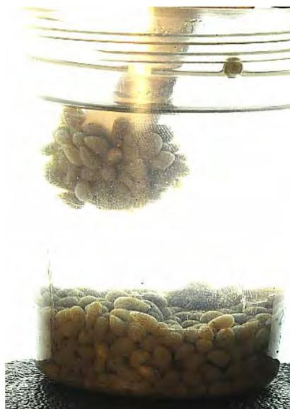
**Figure VI.4: Photograph of 5% iron-cellulose beads in water with a magnet attracting the beads**
