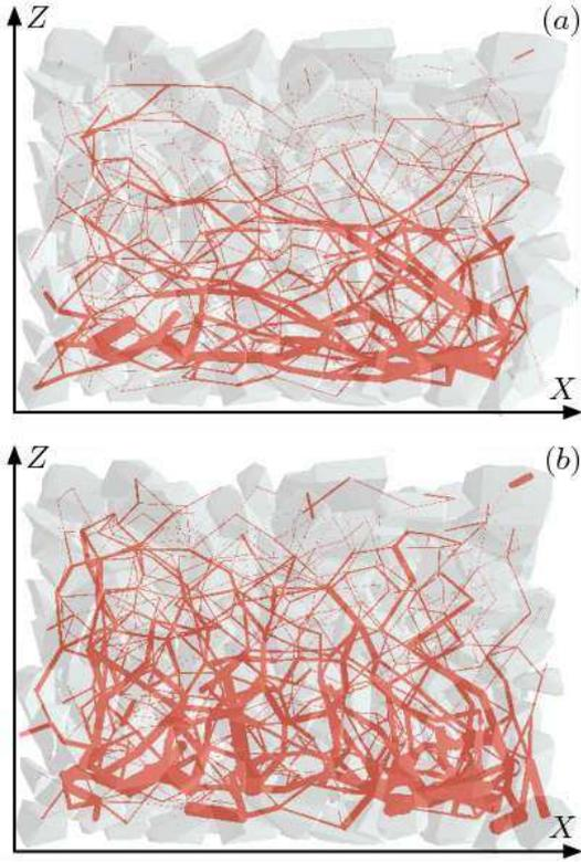
**Fig. 8.** Normal forces in the passive (a) and active (b) states in a section of the packing parallel to the  $xz$  plane. The segments connect particle centers with a thickness proportional to the normal force.
