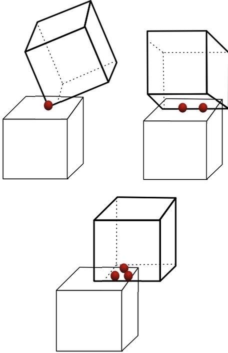
Fig. 1. Different types of contacts between two polyhedra.
