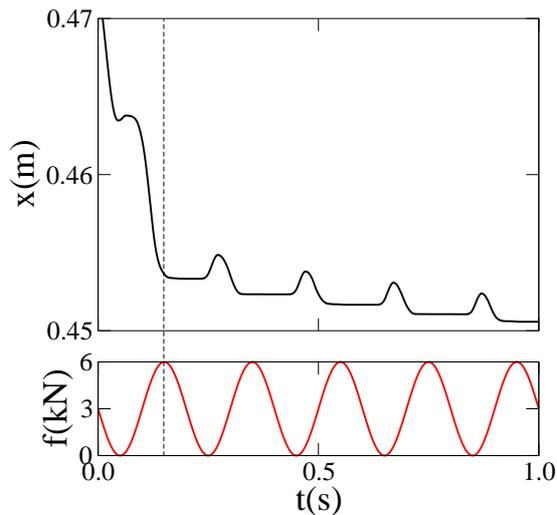
**Fig. 4.** The evolution of the displacement  $x$  of the free wall (up) in response to harmonic loading (down).
