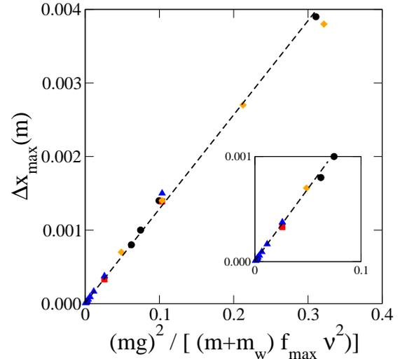
**Fig. 15.** Scaling of the maximum displacement  $\Delta x_{\max}$  with loading parameters from simulations with different values of the frequency  $\nu$  (triangles), the force amplitude  $f_{\max}$  (circles), the gravity  $g$  (squares), and for the mass  $m_w$  (diamonds) of the free wall. The inset shows the plot near the origin.
