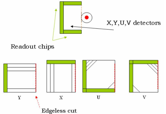
Figure 5: Detector geometries
