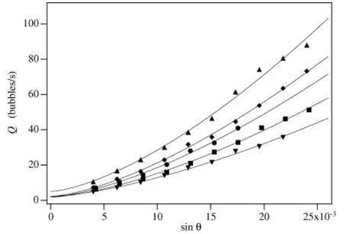
FIG. 4: Bubble flow rate  $Q$  as a function of the tilt angle  $\theta$  of the plane. The curves correspond to different apertures  $D$  of the silo: ( $\blacktriangledown$ )  $D = 6.3$  mm, ( $\blacksquare$ )  $D = 8.0$  mm, ( $\bullet$ )  $D = 9.7$  mm, ( $\blacklozenge$ )  $D = 12.8$  mm, ( $\blacktriangle$ )  $D = 19.9$  mm; (—) best fit of the experimental data with  $Q \propto (\sin \theta)^{3/2}$ .
