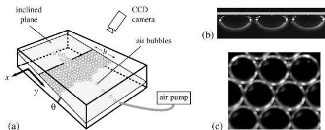
FIG. 1: (a) Sketch of the experimental setup. A transparent inclined plane is immersed into water and tilted at an angle  $\theta$ . Small air bubbles are injected from below at the bottom of the plane and rise towards the top where they aggregate. Motions of the bubbles are recorded by a CCD camera. (b) Side view: the bubbles present an oblate shape. (c) Top view: the bubbles have a circular shape in the bulk.
