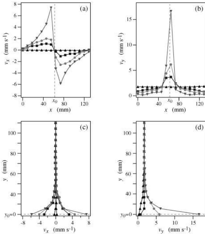
FIG. 2: Transverse  $v_x$  and longitudinal  $v_y$  velocity profiles during the discharge of a silo ( $\theta \simeq 0.63^\circ$ ,  $D \simeq 8.6$  mm). (—) position  $(x_0, y_0)$  of the center of the outlet of the silo. The different curves ( $\blacktriangledown$ ,  $\bullet$ ,  $\blacksquare$ ,  $\blacktriangle$ ) correspond respectively to velocity profiles at increasing distances from  $y_0 = 0$  (Figs. 2a and 2b) and increasing distances from  $x_0$  (Figs. 2c and 2d).
