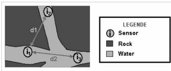
The distance  $d_1$  which separates the sensors  $i_1$  and  $i_2$  is shorter than the distance  $d_2$  which separates the sensors  $i_1$  and  $i_3$ . However, the rock separating the couple of sensors ( $i_1$ ,  $i_2$ ) will degenerate the signal and will prevent sensor  $i_2$  from receiving the message correctly unlike  $i_3$ .
