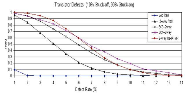
Figure 5. Graph of yield simulator output for WISP-0
