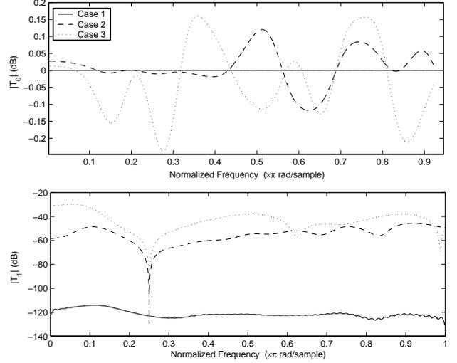
**Fig. 2.** Comparison between the magnitudes of the distortion (high) and aliasing (low) functions in three cases: Case 1 - No analog errors; Case 2 -  $\varepsilon_{R_m} = \varepsilon_{L_m} = 0.01, \varepsilon_{C_m} = 0.005$ ; Case 3 -  $\varepsilon_{R_m} = \varepsilon_{L_m} = 0.05, \varepsilon_{C_m} = 0.01$
