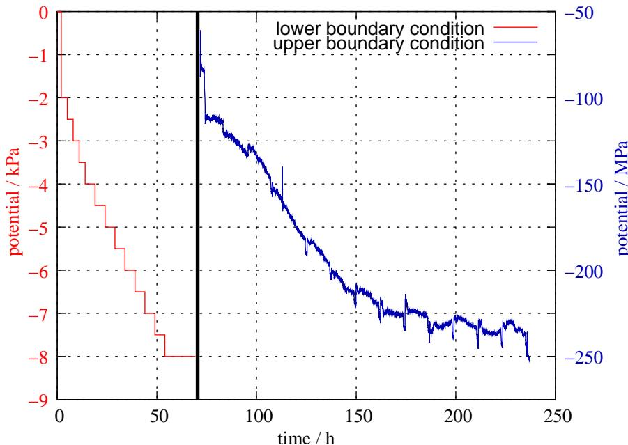
**Fig. 8.** Boundary conditions during the experiment with the sand sample. The red line shows the lower boundary condition during the MSO, the blue line the upper boundary condition during the evaporation experiment. A no-flow boundary condition was set at the upper boundary during MSO and at the lower boundary during evaporation. The black vertical line marks the switch between MSO and evaporation.
