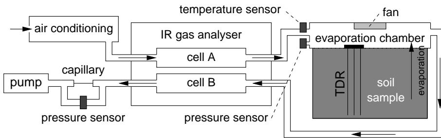
**Fig. 2.** Experimental setup. Evaporation takes place into a gas-tight head space (evaporation chamber) above the soil surface. Air is flowing through it to take away the water. Water vapour molar fraction is measured before and after the head space. The air is conditioned before it enters the chamber to set a well defined boundary condition. The gas flow is measured with a capillary and controlled with a vacuum pump with adjustable speed.
