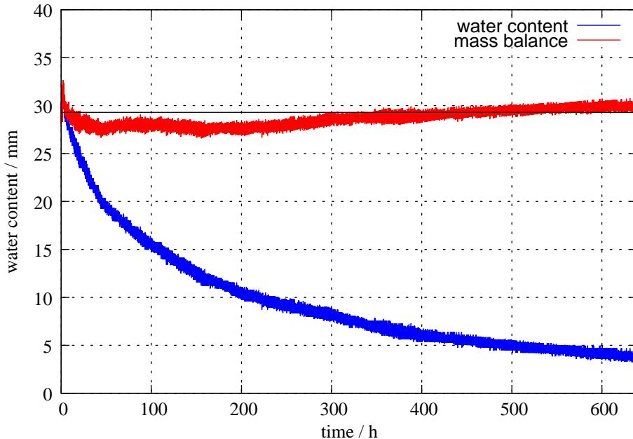
**Fig. 12.** Total water content of the Grenzhof soil sample, measured by TDR (blue), and the mass balance  $\eta\theta_i(t) + \int_0^t j_{\text{exp}}^w(\tau)d\tau$  (red). The black horizontal line represents the initially measured water content.
