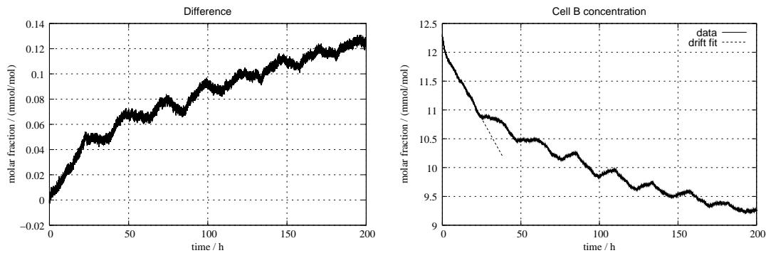
**Fig. 3.** Water vapour molar fraction measurements of the gas analyser with conditioned air at 10°C dew point flowing simultaneously through both cells of the instrument. The difference (left) is very stable while the absolute molar fraction (right) is drifting faster, with about  $-49 \mu\text{mol mol}^{-1} \text{ h}^{-1}$  on the first day (dashed line).
