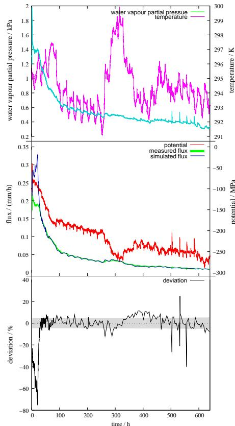
**Fig. 11.** Results of the evaporation experiment with the Grenzhof soil sample. Notice that measured and simulated flux (middle frame) practically overlap. The relative deviation  $(j_{\text{exp}}^w - j_{\text{model}}^w)/j_{\text{exp}}^w$  is shown in the bottom frame together with the measuring uncertainty from Fig. 13 (gray band).
