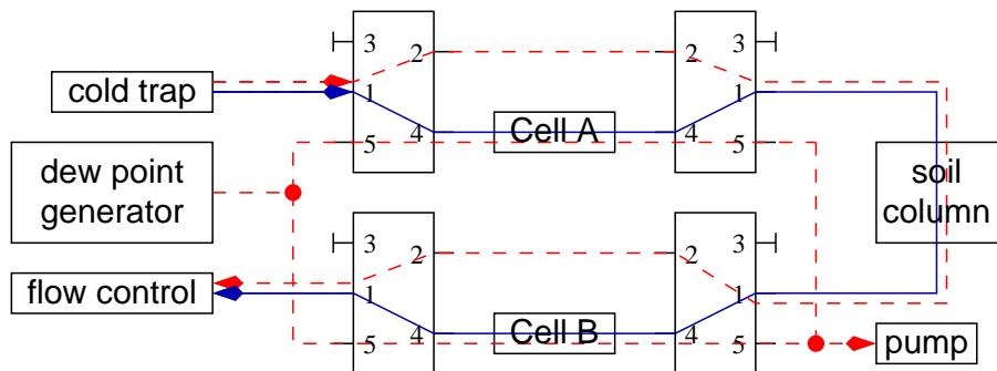
**Fig. 5.** Setup for runtime calibration. In normal operation (blue line), all valves are in state (1). During calibration (red dashed lines), the four valves are set to state (2), the measured gas bypasses the gas analyser and conditioned air from the dew point generator is flowing through both cells.
