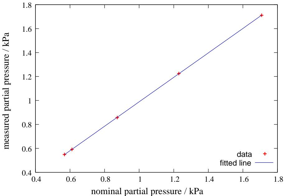
**Fig. 4.** Linearity and calibration check of the gas analyser. Null gas was flowing through cell A and air with defined water vapour molar fraction through cell B. The nominal cell B molar fraction was varied and the measured partial pressure  $p_{\text{meas}}$  recorded.
