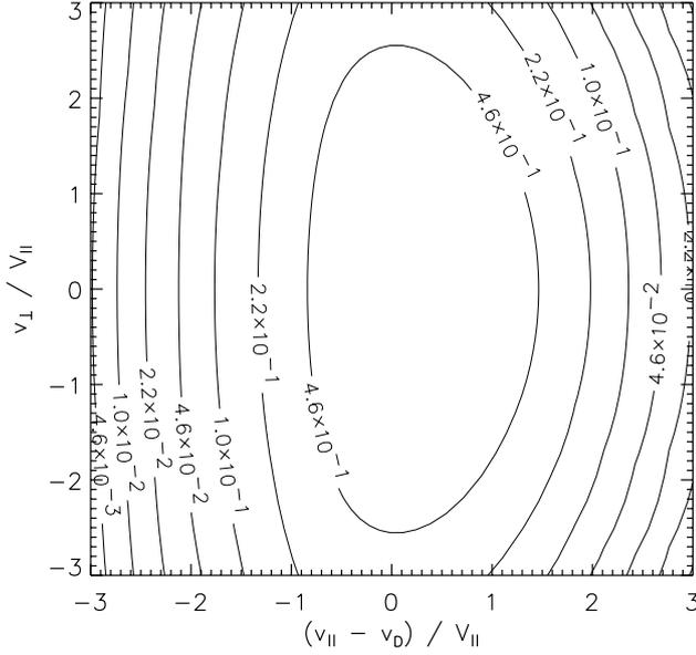
**Fig. 5.** Two-dimensional gyrotropic model VDF of  $O^{5+}$  ions at  $1.44 R_{\odot}$ , displaying a distinct kinetic temperature anisotropy and skewness (heat flux) away from the Sun (Vocks and Marsch, 2002b).
