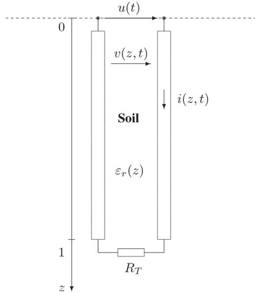
Fig. 1. Schematic view of the TDR line.
