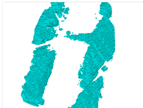
Fig. 3. Visual Hull reconstructed by shape-from-silhouette with regular voxelization and SPOT projection test
