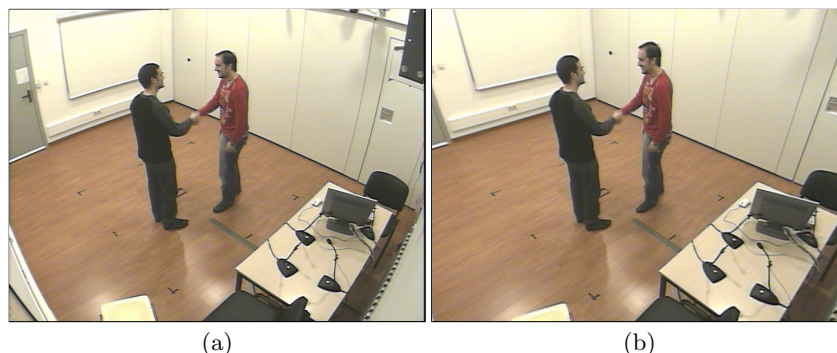
Fig. 1. A captured image as seen from one of the cameras (a) and its corresponding undistorted version (b)
