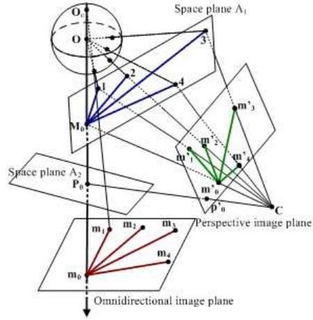
Fig. 2. Relationship between omnidirectional and perspective image points
