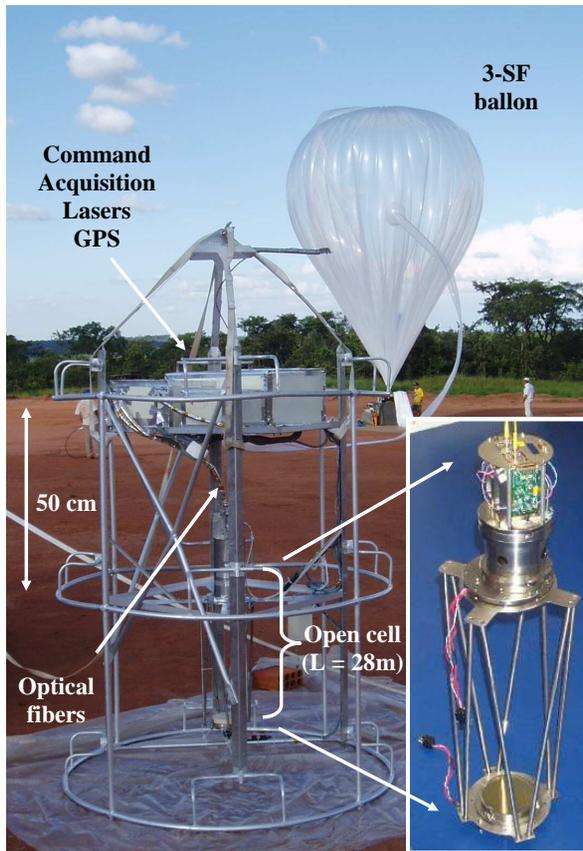
**Fig. 1.** The micro-SDLA diode laser spectrometer during HIBISCUS in Bauru, Brazil in February 2004. With an overall weight of less than 40 kg, the micro-SDLA sensor is flown from small-size 3000 m<sup>3</sup> balloons to reach a float altitude near 22 km.
