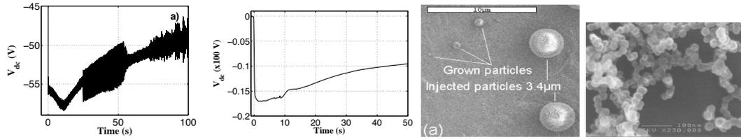
**FIGURE 1.** From the left to the right: evolution of the self-bias voltage during the dust particle growth in the PKE-Nefedov reactor; Evolution of the self-bias voltage during the dust particle growth in the ComPLEXS reactor; dust particles collected in the PKE-Nefedov reactor; dust particles collected in the ComPLEXS reactor
