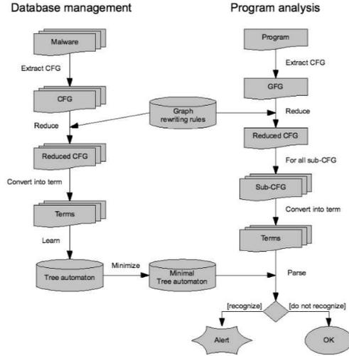
Figure 1: Design of the control flow detector
