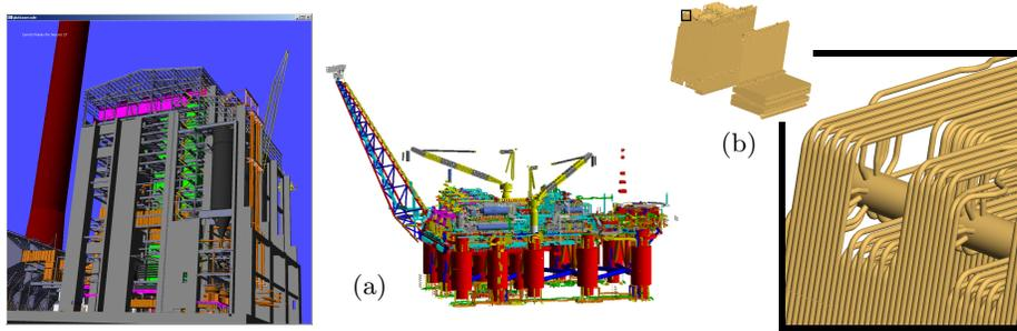
**Fig. 6.** (a) PowerPlant and P40 Oil-Platform models used on performance tests. (b) PowerPlant Section 1, about 60,000 primitives recovered from 3,500,000 triangles. The thickness control prevents undesired visible patterns when cylinders are seen from far.
