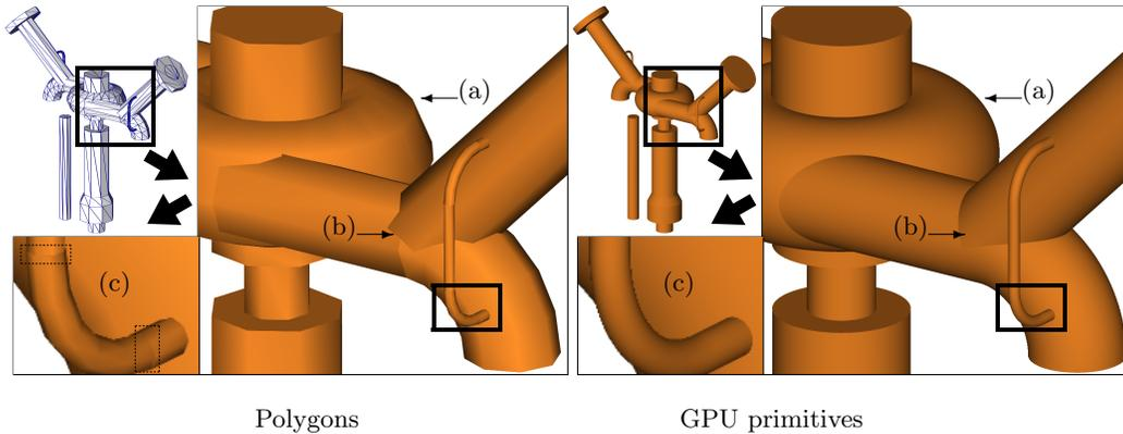
**Fig. 1.** An industrial piece in PowerPlant (section 13). *Left:* Original tessellated data. *Right:* Rendering with implicit GPU primitives. *Image quality enhancement:* (a) silhouette roundness; (b) precise intersection; (c) continuity between consecutive primitives.
