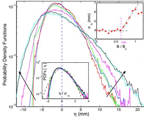
FIG. 5: Probability density functions of wave amplitude,  $\eta$ , for different values of the dimensionless magnetic induction, from  $B/B_c = 0, 0.3, 0.54, 0.77, 0.92$  to  $1.2$  (see the arrows). Forcing parameter:  $1 \leq f \leq 4$  Hz. Bottom inset: Same PDFs displayed using the reduced variable  $\eta/\sigma_\eta$ . Gaussian fit (dashed line). Top inset: Standard deviation of wave amplitude  $\sigma_\eta$  as a function of  $B/B_c$ .
