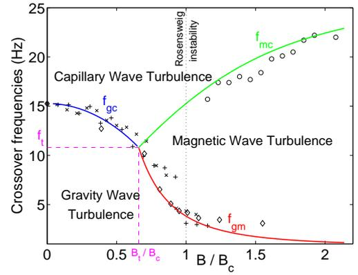
FIG. 4: Rescaled crossover frequencies,  $\tilde{f}(B) \equiv f_{gc}(0) \times f(B)/f(0)$  as a function of  $B$  for different frequency bandwidths of the random forcing: (x) 1 to 4 Hz, (◊) 1 to 5 Hz, and (+ or o) 1 to 6 Hz. Theoretical curves  $f_{gc}$ ,  $f_{gm}$  and  $f_{mc}$  are respectively from Eqs. (5), (6) and (7). The triple point ( $f_t = 10.8$  Hz,  $B_t/B_c = 0.65$ ) is from Eq. (8).
