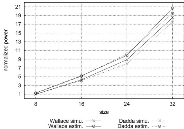
Fig. 6. Power estimation results compared to Spice simulations
