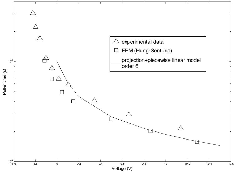
**Figure 2** - Pull-in time (s) versus applied voltage (V) for  $P_0=1.013\times 10^5$  Pa. Comparison of the experimental and simulated results presented in [16] to the simulated results obtained with our reduced-order model. The chosen squeeze modes correspond to  $k_1=0, 2$  and  $k_2=1, 3$  in (38). For the mechanical part, the first eigenmode is used.
