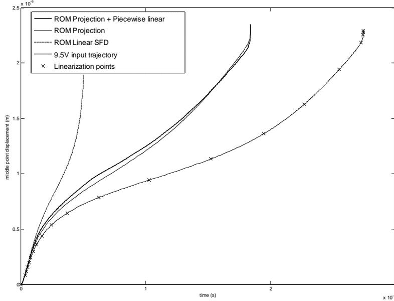
**Figure 1-** Middle point displacement of a microswitch for a linear model, the projected model and the projected and piecewise linearized model (1 mechanical mode, 4 squeeze modes) for a 10V step voltage. The 21 linearization points are chosen along a 9.5V input trajectory.
