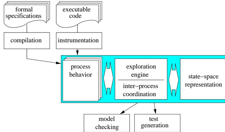
**Fig. 1.** Functional view of IF-2.0 exploration platform.
