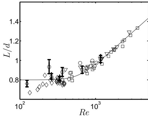
FIG. 8: Dependence of  $L/d$  versus  $Re$  for both cells. Same symbols as in figure 7. The line correspond to a fit of our data with the formula:  $(L/d) = 0.075 \ln(1 + (Re/Re^*)^4) + 0.8$ , with  $Re^* = 600$ .
