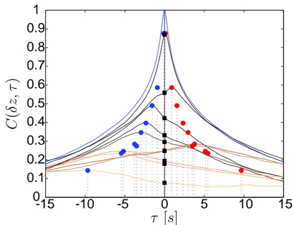
FIG. 3: The correlation function  $C(\delta z, \tau)$  for various  $\delta z$  in the high power case (235W). The dots correspond to the position of the highest peak and its symmetric compared to  $\tau = 0$ . The squares mark the value of  $C(\delta z, 0)$  for the different  $\delta z$ , from the darker to the lighter: 4mm, 10mm, 20mm, 30mm, 40mm, 50mm (twice), 60mm, 70mm, and 100mm. The blue (top) curve corresponds to the autocorrelation of one sensor (*i.e.*  $\delta z = 0$ ).
