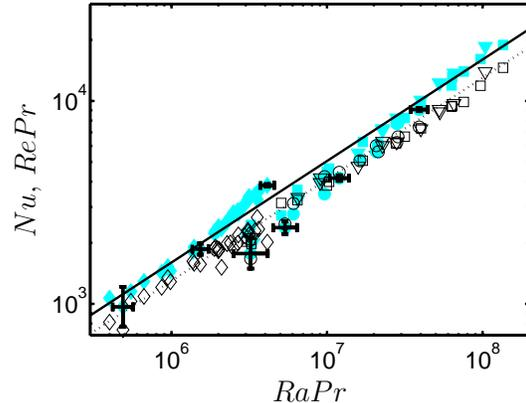
FIG. 7: Evolution of  $Nu$  (full symbols) and  $RePr$  (open symbols) *versus*  $RaPr$ . First cell:  $\circ$ ,  $Pr = 6.6$ ;  $\nabla$ ,  $Pr = 5.3$ ;  $\square$ ,  $Pr = 4.1$ . Second cell:  $\diamond$ ,  $Pr = 6$ . Full line, proposed average law for  $Nu$  results:  $Nu = 1.6\sqrt{RaPr}$ . Dotted line, proposed average law for  $RePr$  results:  $RePr = 1.3\sqrt{RaPr}$
