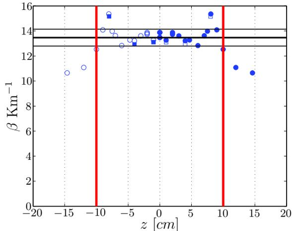
FIG. 6: Temperature gradient *versus* the height in the cell, for the second cell. Only full symbols correspond to real measurements. Open symbols are simply symmetric to the full ones compared to the middle of the cell. The two vertical bars signal the ends of the channel. The thick horizontal line stands for the average of  $\beta(z)$  in the center of the channel. The lower and upper horizontal lines correspond to  $\pm 5\%$  of this mean value.
