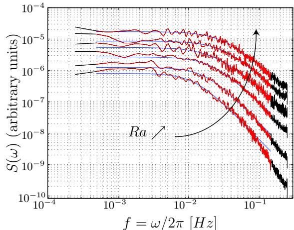
FIG. 5: The spectra of the bridge output, for various  $Ra$  values (second cell,  $Pr = 6$ ). The lines correspond to the fit used for extracting  $\tau_o$ . The range for the fit is signaled in red on the spectrum.
