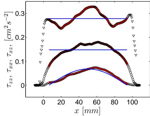
FIG. 13: The Reynolds stresses  $\tau_{xx}$  ( $\circ$ ),  $\tau_{zz}$  ( $\nabla$ ), and  $\tau_{xz}$  ( $\triangle$ ), versus  $x$ , for the lowest power (93W). The full symbols correspond to the range of the fit ( $x_- = 7\text{mm}$ ,  $x_+ = 94\text{mm}$ ). The lines show the proposed fit.
