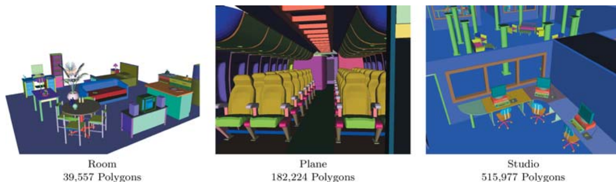
Fig. 7. Scenes used for testing the object congruency descriptor. In each scene, the descriptor has been used to detect objects with similar geometry (but possibly different meshes) up to a rigid transform. Objects found to be congruent are displayed with the same color.
