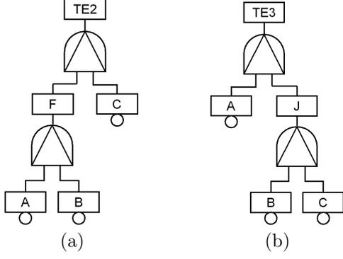
Fig. 4. Basic PDFTs made of a cascade of PAND gates
