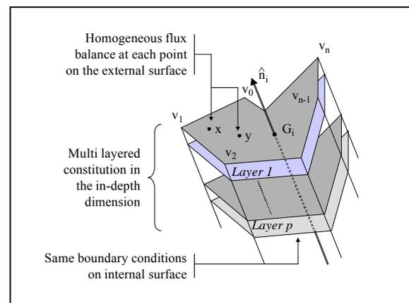
**Figure 1—The multi-layered in-depth constitution of an element.**
