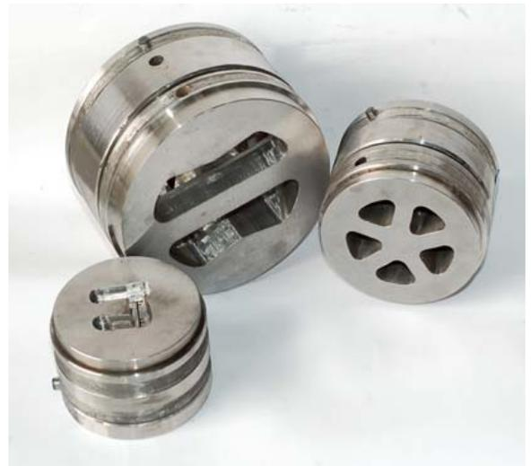
Figure 9: Aluminum extrusion dies
