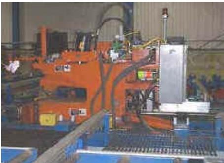
Figure 7: Extrusion cut-off saws
