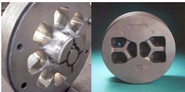
Figure 13: Typical hollow dies
