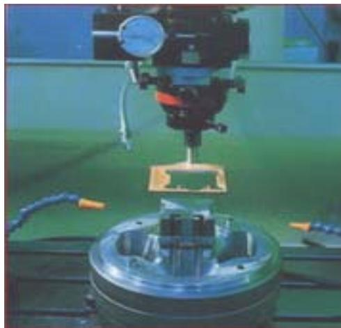
Figure 24: EDM sparking process
