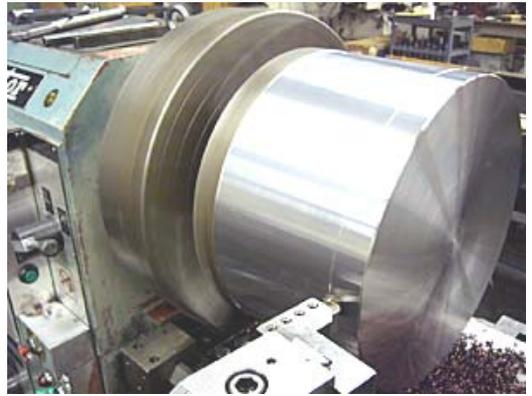
Figure 21: Turning operation
