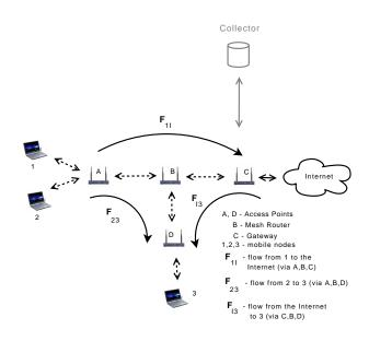
Fig. 2: Wireless Mesh Network – flow example
