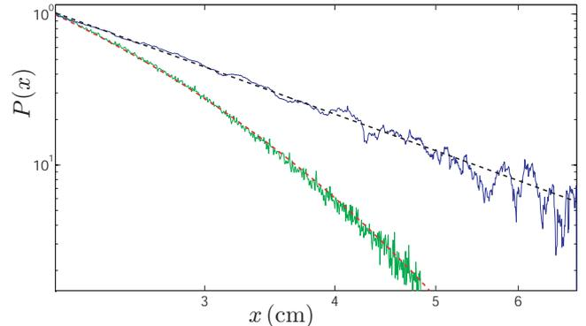
**Fig. 2.** Experimental measurements of the step size distribution function (log-log scale) in the configuration of Figure 1(a) and (b). With an incident laser beam (green crosses), the observed decay is well fitted by an exponential (red dotted line) as expected from Beer-Lambert law. In the two-cell configuration, the data (continuous blue line) are well fitted by a power law (black dotted line)  $P(x) = 1/x^\alpha$ , with  $\alpha = 2.41 \pm 0.12$ .
