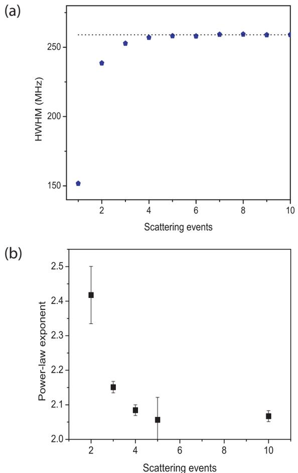
**Fig. 4.** Evolution of (a) the HWHM of the photons spectral distribution and (b) the power-law exponent  $\alpha$ , with the number of scattering events in a Rb vapor at 300K. The original spectral distribution (photons absorbed in the zeroth order diffusion) is the one of a resonant, monochromatic laser.
