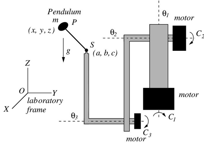
Figure 4: The robot  $2k\pi$  carrying its pendulum.
