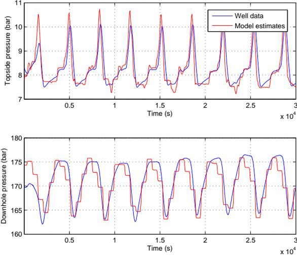
Fig. 8. Comparison between the observer estimates for  $k = 0.05$  and the real measurements. After only one oscillation, the system is perfectly synchronized in terms of frequency and amplitude. The observer allows to reconstruct the downhole pressure from topside measurements.
