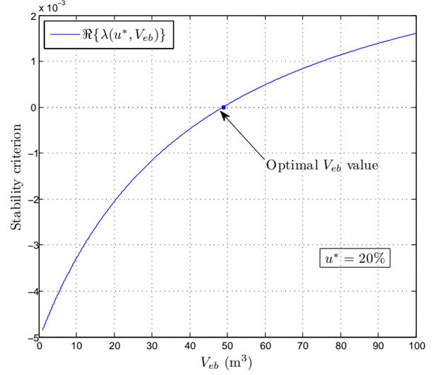
Fig. 2. Value of  $\Re\{\lambda(u^*, V_{eb})\}$  as  $V_{eb}$  increases. When the eigenvalues cross the imaginary axis, the criterion is exactly 0. The corresponding value of  $V_{eb}$  should be used in the model.
