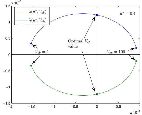
Fig. 3. Locus of the eigenvalues  $\lambda(u^*)$  and  $\bar{\lambda}(u^*)$  when  $V_{eb}$  varies. For low values of  $V_{eb}$ , the eigenvalues are in the LHP. As the parameter increases, the eigenvalues cross the imaginary axis, which corresponds to the criterion plotted in Figure 2 being 0.
