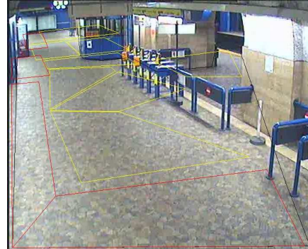
Fig 4. The yellow polygons show the outline of the learned lost zones. The red polygons show the outline of the entry zone, exit zone and IO zones.
