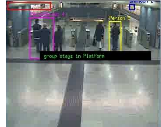
Figure 2.10 Group of persons staying in the hall (biggest bounding box) and a luggage (smallest bounding box) erroneously detected.
