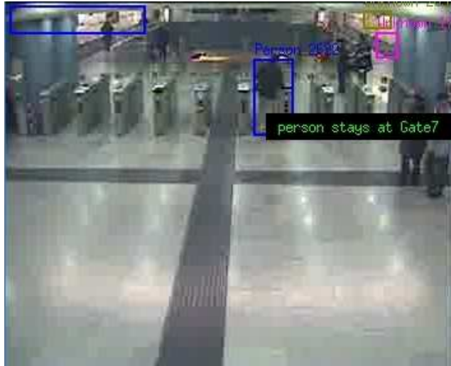
Figure 2.8 Person detected staying at gate 7 (biggest bounding box).
