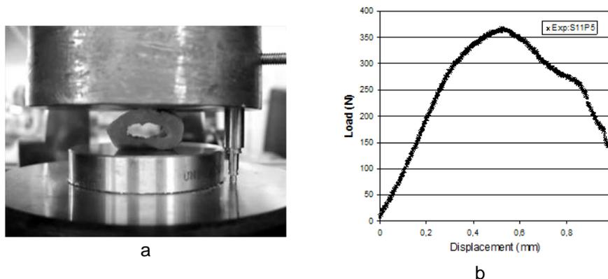
Fig. 4 - Mechanical test; (a) Compression test using an LVDT extensometer, (b) Load vs. Displacement curve
