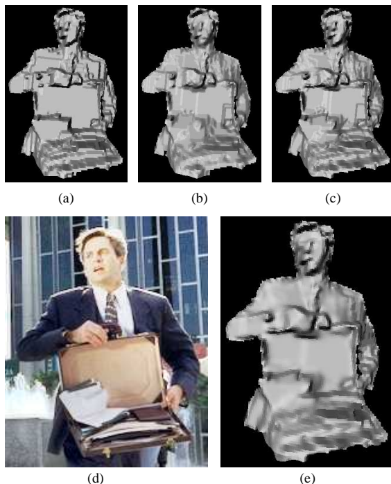
Figure 7: 3D reconstructions with various parameters (a) Without PDE filter and with a linear smoothing term: spurious discontinuities (on the shoulders and on the arms) (b) Without PDE filter and discontinuity maps: details are blurred (on the face and in the briefcase) (c) Without PDE filter: aliasing. (d) An input image. (e) Final result with all our contributions.
