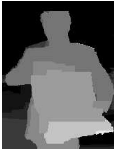
Fig. 16. Disparity map computed with the method of Kolmogorov et al. [1] on the same sequence as Figure 14.
