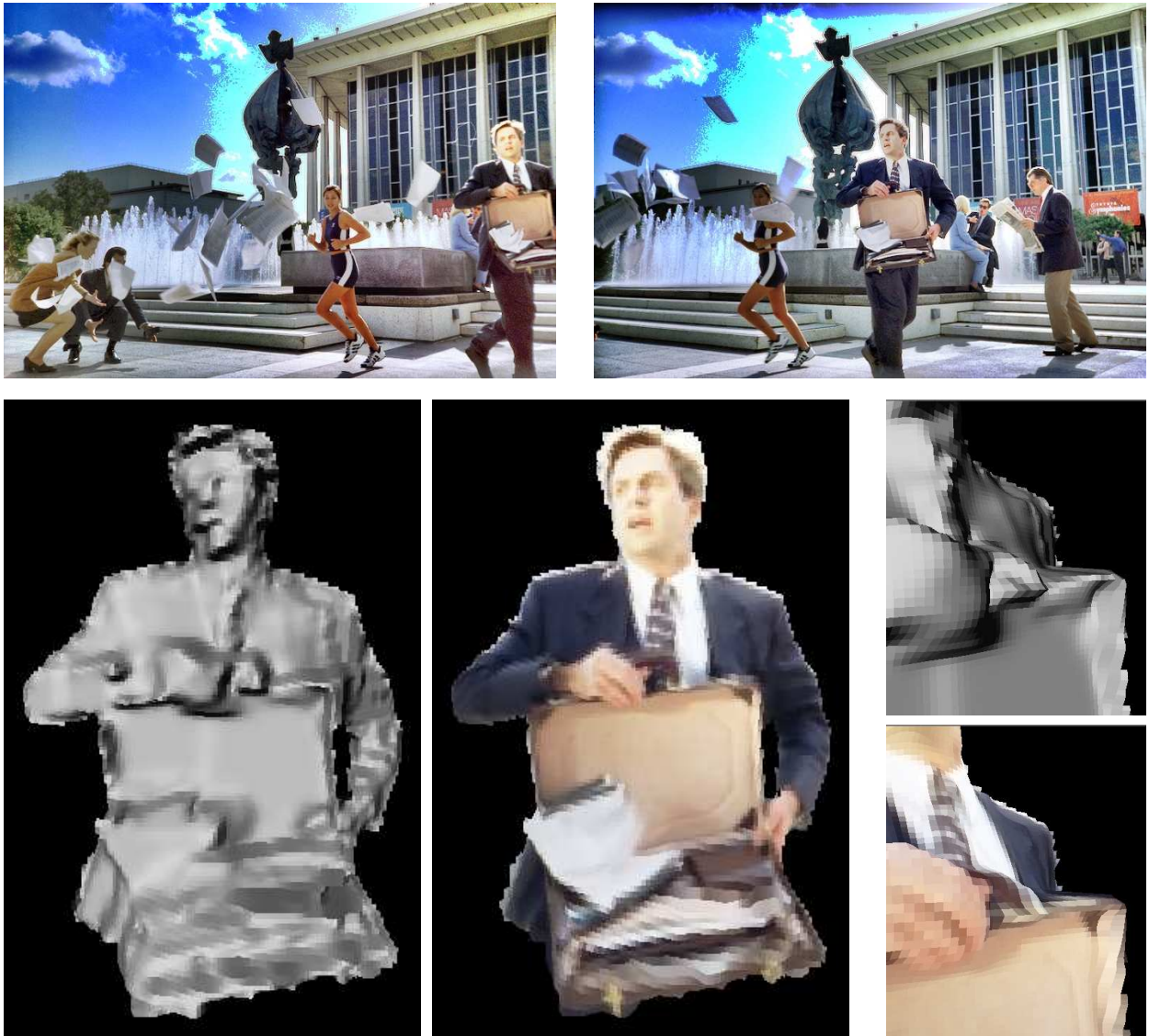
Fig. 14. Man with briefcase reconstruction (right) 40 images at 692 \times 461 , face is about 40 \times 40 (left). Notice that the discontinuities are preserved.
