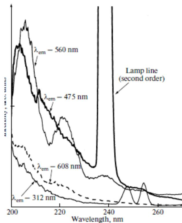
**Fig. 2.** Photoluminescence excitation spectra of the aluminoborosilicate glass doped with  $Gd^{3+}$  ions (0.88 mol %) in the range of emission of defects at the wavelengths  $\lambda_{em} = 475$ , 560, and 608 nm. For comparison, the photoluminescence excitation spectrum of the band of  $Gd^{3+}$   $\lambda_{em} = 312$  nm for the same sample is shown.
