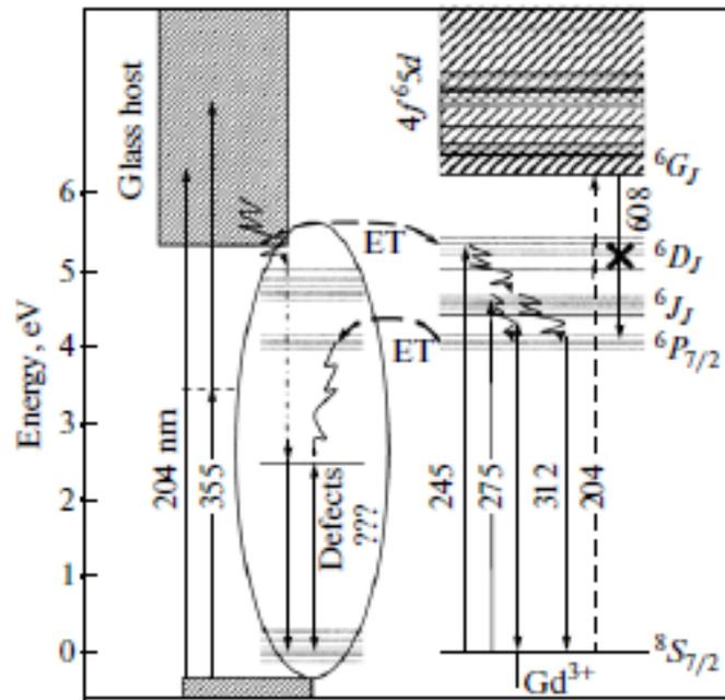
**Fig. 6.** Scheme of the levels of a  $Gd^{3+}$  ion and a model describing the mechanisms of energy transfer (ET) and origin of the luminescence in the aluminoborosilicate glass doped with  $Gd^{3+}$  ions. The transition shown by the thick dashed arrow corresponds to band–band absorption of the aluminoborosilicate matrix, and the transition marked by the cross is not observed in the glass under investigation.
