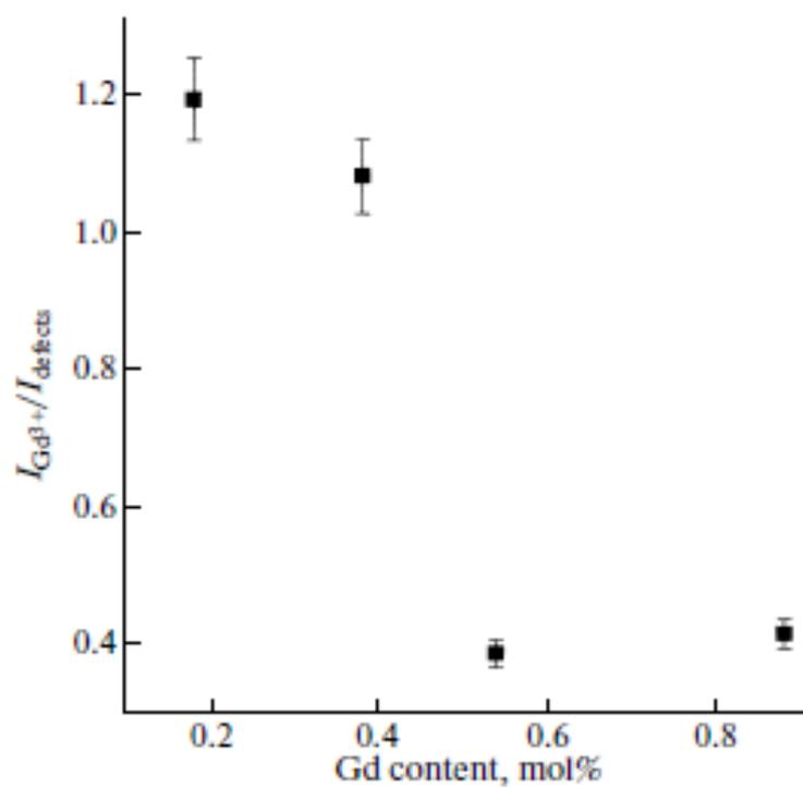
**Fig. 5.** Relationship between the intensities of the luminescence bands of  $Gd^{3+}$  ions and optically active defects of the aluminoborosilicate glass for different gadolinium concentrations ( $\lambda_{ex} = 355$  nm, Nd : YAG laser).
