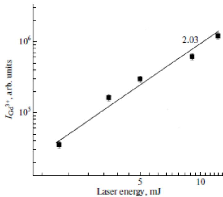
**Fig. 4.** Dependence of the intensity of the luminescence band at 312 nm  $I_{\text{Gd}^{3+}}$ , on the intensity of exciting light with  $\lambda_{\text{ex}} = 355$  nm. The number in the graph indicates the slope of the straight line on a double logarithmic scale.
