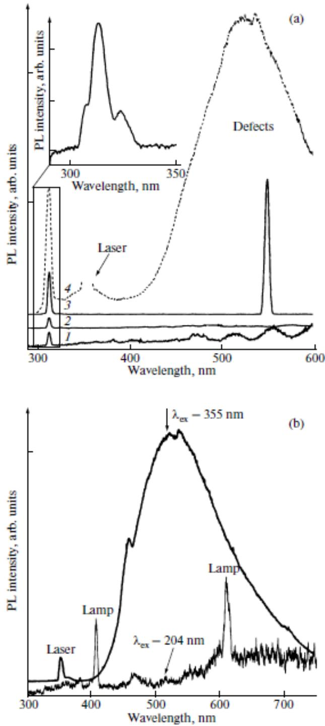
**Fig. 1.** Photoluminescence spectra under excitation by light with different wavelengths  $\lambda_{\text{ex}}$ : (a) aluminoborosilicate glass doped with  $\text{Gd}^{3+}$  ions (0.88 mol %) and (b) undoped aluminoborosilicate glass.  $\lambda_{\text{ex}} =$  (1) 204 nm (Xe lamp), (2) 245 nm (Xe lamp), (3) 275 nm (Xe lamp), and (4) 355 nm (Nd : YAG laser). The inset shows the spectral portion corresponding to the  ${}^6P_{7/2} - {}^8S_{7/2}$  optical transition of the  $\text{Gd}^{3+}$  ion.
