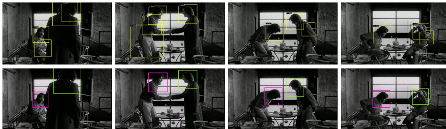
Fig. 2. Upper body detections (top row) and tracks (bottom row) after classification post-processing for a sample test sequence of CEC . The bounding box colours indicate different tracks. Note the improvement due to the tracking where false positives have been removed, as well as the high accuracy despite motion, articulations and self-occlusions.
