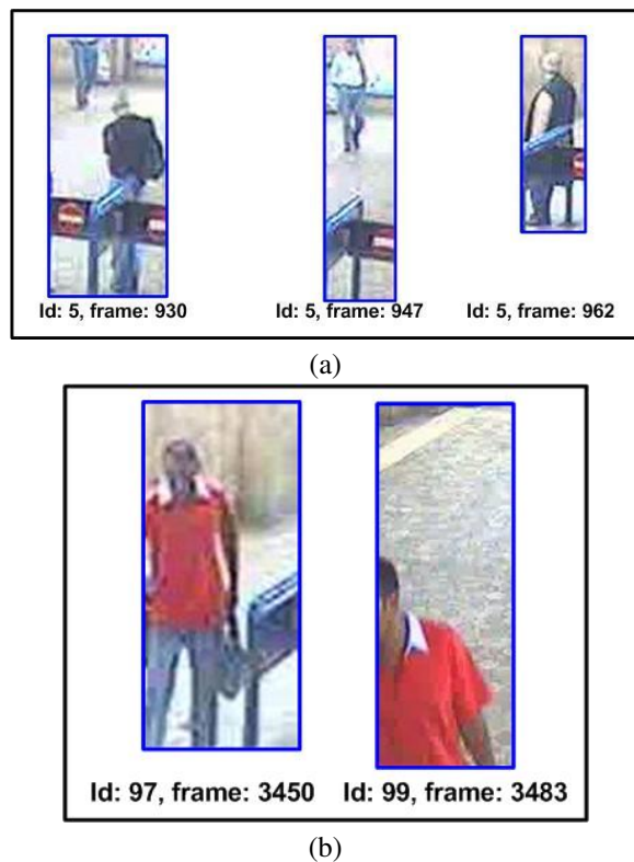
Fig. 4. (a) three ground-truth objects IDs associated to one sole detected object (object ID confusion = 3); (b) two tracked objects created for one sole ground-truth object (object ID persistence = 2).
