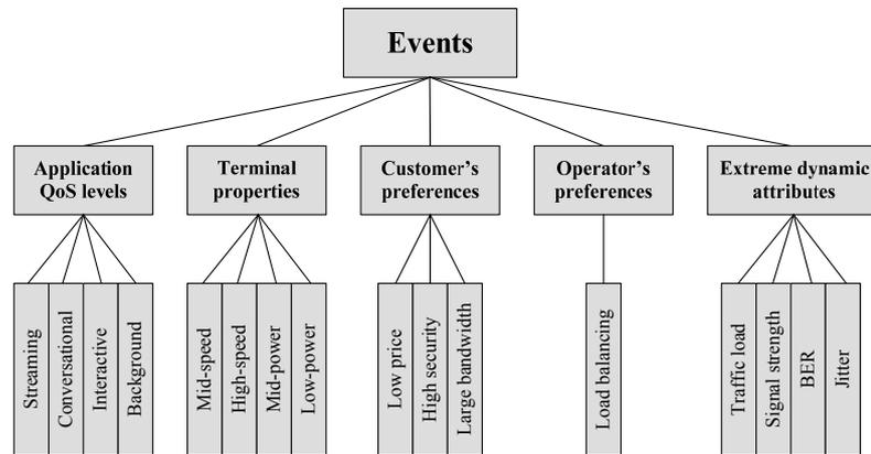
**Figure 5- 1 Hierarchy of trigger events.**
