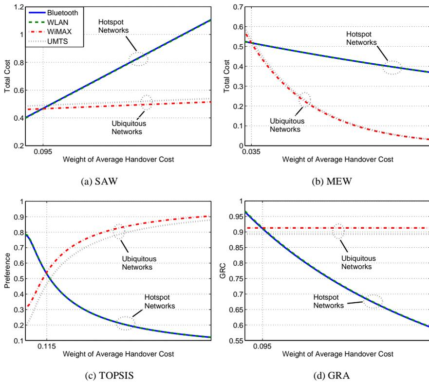
Figure 4- 8 Coefficients of various networks vs. Weights of average handover cost.
