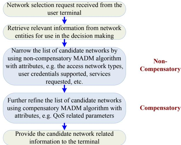
**Figure 2- 19 Compensatory and non-compensatory integrated network selection.**
