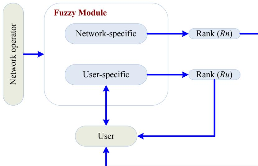
**Figure 2- 26 Network specific and user specific combined network selection.**
