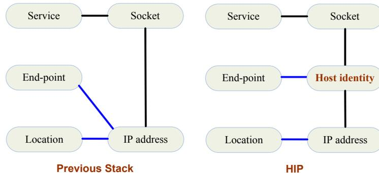
Figure 2- 6 Host identity protocol stack.
