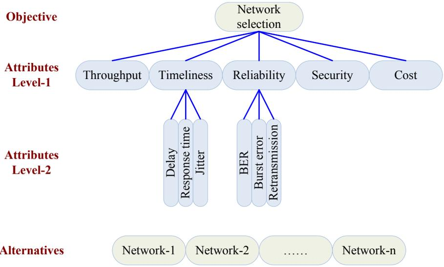
**Figure 2- 21 An example of an AHP hierarchy of criteria.**
