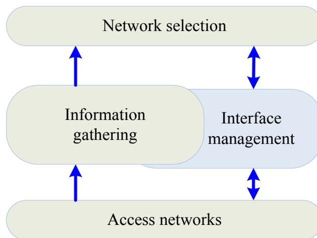
**Figure 2- 28 Terminal-controlled network selection scheme.**
