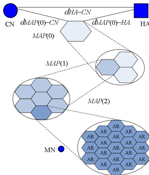
Figure 6- 1 A three-layer MAP model for HMIPv6 networks.
