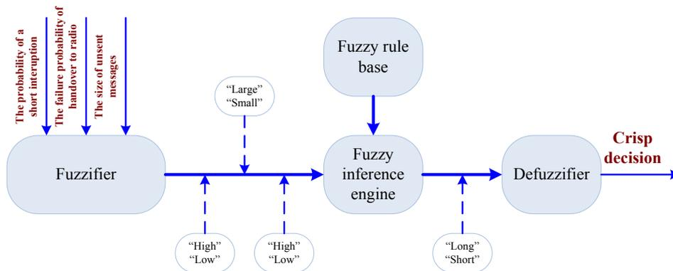
Figure 2- 23 The procedure of fuzzy logic based VHO decision.
