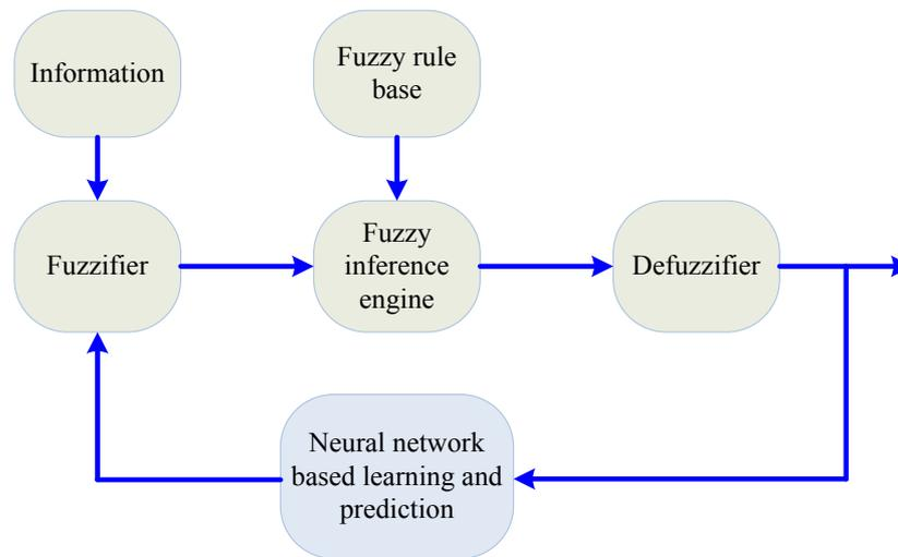
**Figure 2- 27 Network selection combining fuzzy logic and neural network.**
