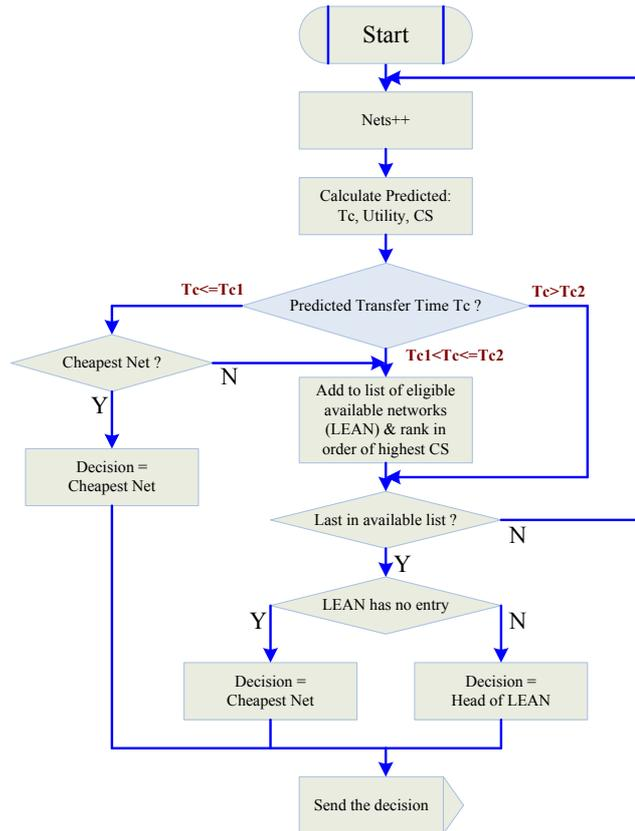
**Figure 2- 18 A utility-based network selection strategy focusing on transfer time cost.**
