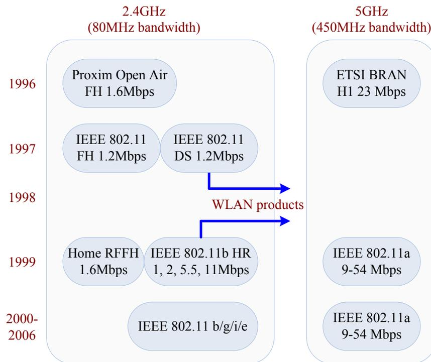
**Figure 2- 3 The evolution of WLAN standards.**
