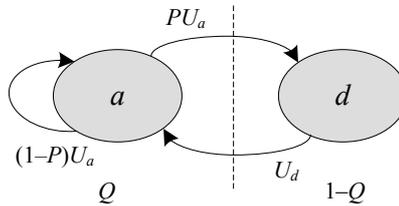
**Figure 4- 6 Transition of an MT within 2 states.**
