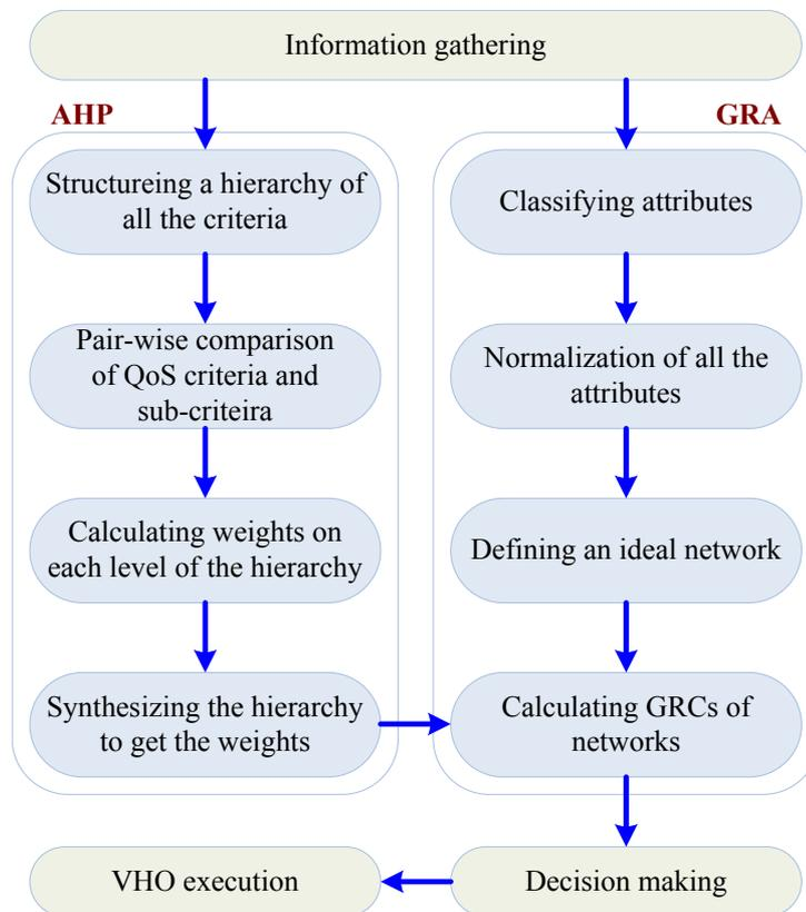
**Figure 2- 20 Combined procedure of AHP and GRA.**
