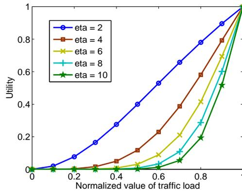
Figure 7- 1 Utility function for traffic load.
