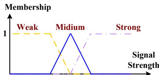
Figure 2- 22 Membership function of ‘signal strength’.
