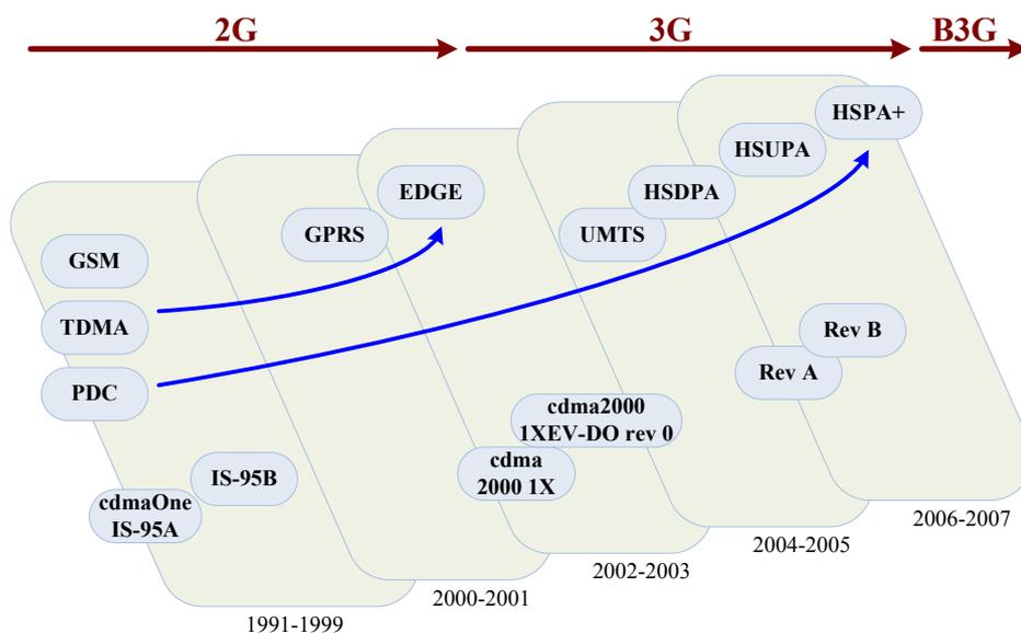
Figure 2- 2 The evolutionary of WWAN technologies [LP08].
