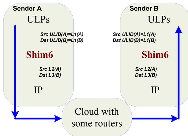
Figure 2- 7 Mapping with changing locators in shim6.
