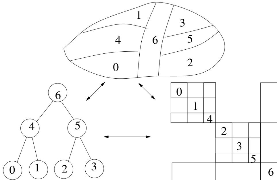
Figure 1: Graph partitioned into 4 parts, its corresponding separator tree and matrix obtained after re-ordering.
