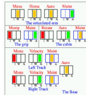
Fig. 5. The model of the excavator tasks.
