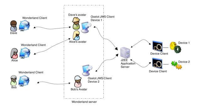
Let's take a scenario for better understanding what are the role and aims of each software brick. Suppose that you have two devices, which are remotely controlled through the J2EE Remote lab framework (called OCELOT). Each of them
