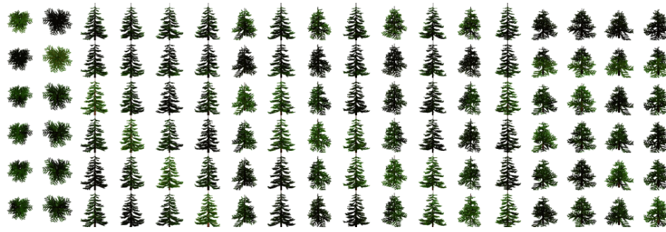
Fig. 6. The BTF associated to the highest level (horizontal axis: 18 view directions, vertical axis: 6 light directions, 64 \times 64 resolution per billboard, with colors and transparencies).
