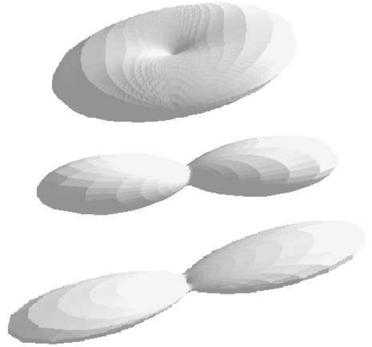
Fig. 18. Normals distribution function (NDF) of various ellipsoids. The radius are, from top to bottom: 1 \times 1 \times 2 , 1 \times 2 \times 2 , 1 \times 2 \times 4 . To be noted that the absolute size has no meaning: each distribution has to be normalized so that the integral is 1 (thus the NDF can be seen as the probability to get a normal in a given direction).
