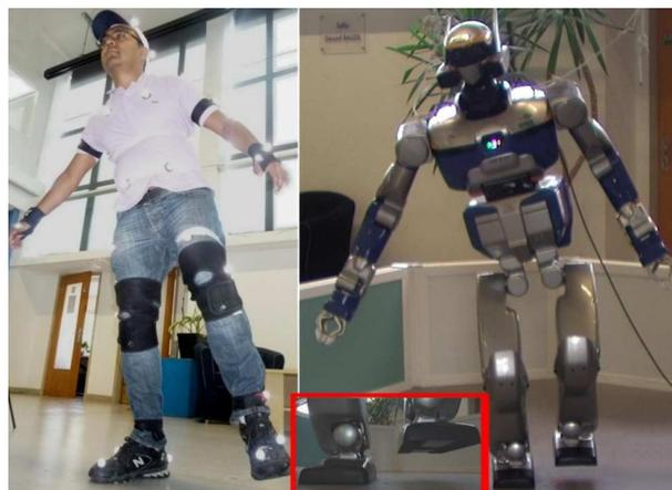
Figure 4.6: Scenario 2. Picture of humanoid imitating the human lifting his foot.
